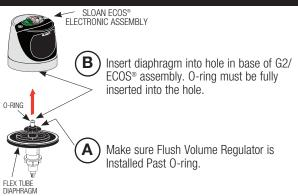
Push Diaphragm securely against underside of Sloan ECOS® Electronic Assembly. Place entire Assembly onto the Valve Body.
