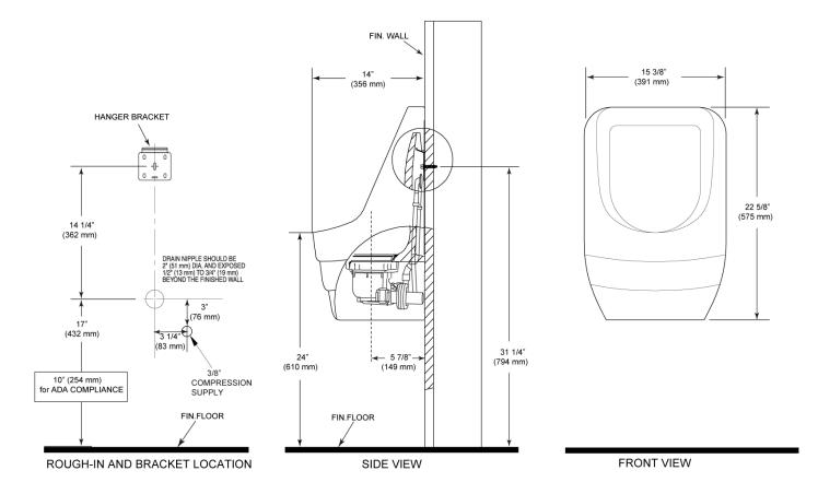
NOTE: ADA urinal rim height requirements allow all heights 17" and below. Sloan strongly recommends roughing in the drain to achieve a 16<sup>1</sup>/<sub>2</sub>" rim height or less to ensure compliance.
